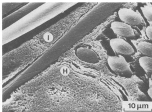
**Figure 4** SEM micrograph of industrially prepared carbon composite after 2 h oxidation in chromic acid.
