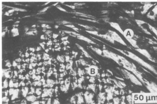
Figure 1 Optical micrograph of CFRC BB-UHT.
