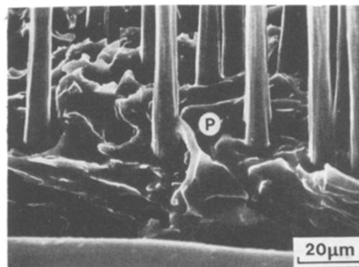
Figure 9 SEM micrograph of HTU fibres in an A240 matrix after 7 h oxidation in chromic acid.
