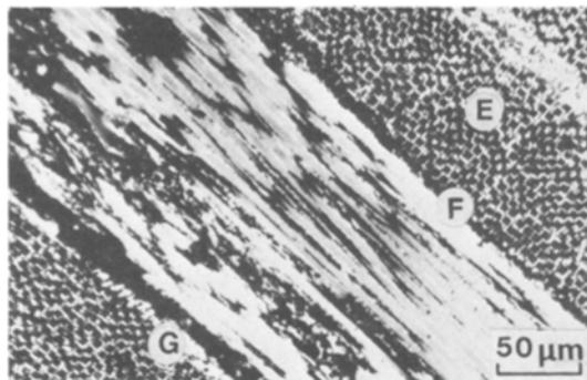
**Figure 3** Optical micrograph of industrially prepared carbon composite.
