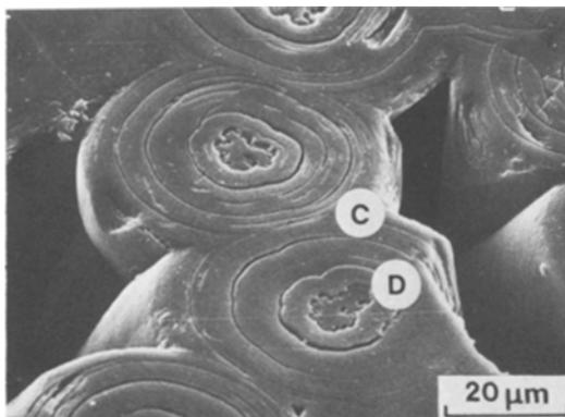
Figure 2 SEM micrograph of a polished surface of CFRC BB-UHT after 4 h oxidation in chromic acid.
