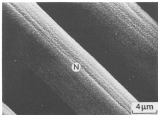
Figure 7 SEM micrograph of CVD coated PAN fibre.
