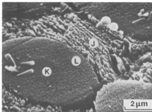
**Figure 5** SEM micrograph of industrially prepared carbon composite after 2 h oxidation in chromic acid.
