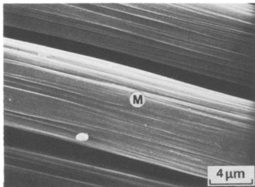
Figure 6 SEM micrograph of HTU PAN fibres.
