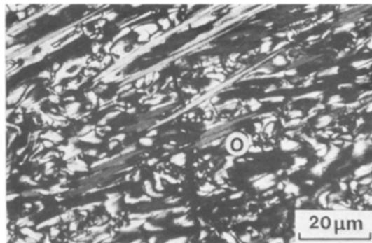
Figure 8 Optical micrograph of HTU fibres in an A240 matrix. HTT 1173 K,  $3 \text{ K min}^{-1}$ .
