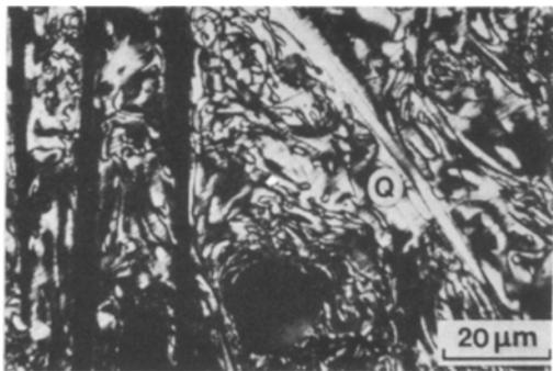
**Figure 10** Optical micrograph of CVD coated fibres in an A240 matrix. HTT 1173 K, 3 K min<sup>-1</sup>.
